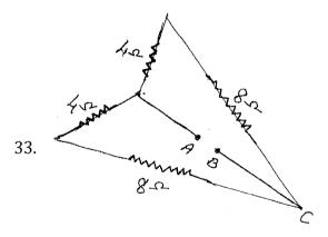
The equivalent resistance between the points A and B shown in the above figure is
